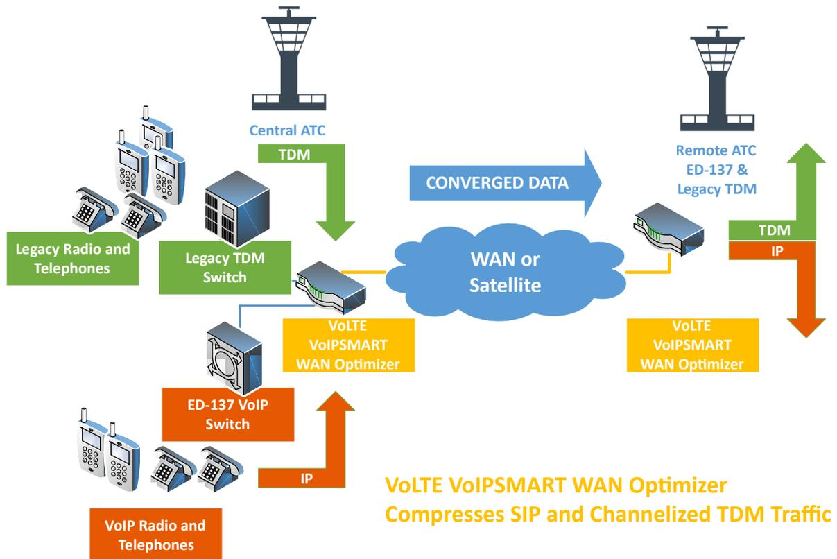
As this compression technique allows the transmission of VoIP and TDM voice over the same WAN circuits in a single converged network, it allows ATC organizations to move to VoIP at their own pace, whilst maintaining their existing equipment and still benefitting from cost reduction through a single converged network. The **VoLTE VoIPSTART** solution adheres to EUROCAE ED-137 ensuring compatibility with all the equipment implemented within the network.
