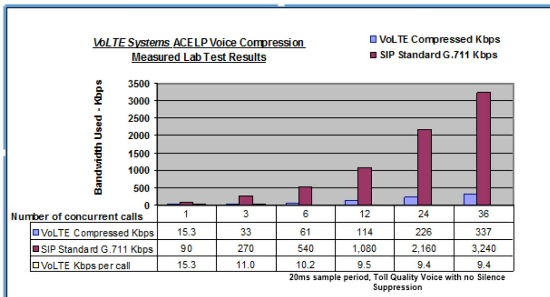
The exact performance gain is dependent on the sample periods being compared. The graph above shows that for 12 or more simultaneous calls the total bandwidth used by SD-VOICE compared with standards based G.711 SIP calls using a 20ms sample period is approximately 9:1. By contrast, if a 10ms SIP sample period is used the advantage is over 11:1 (not shown).
