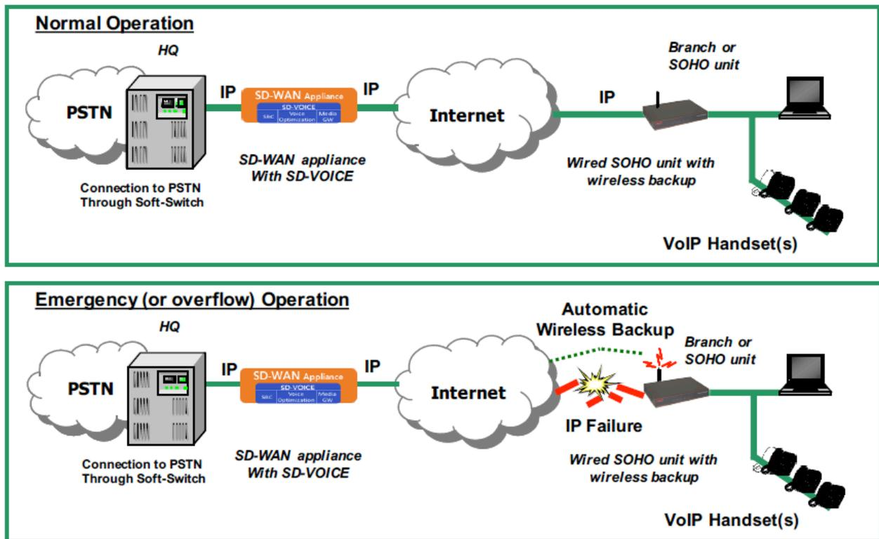
Alternatively, SD-VOICE can also be used to bypass a local PSTN line failure using existing IP network connections and the unique TDM over IP fail-over capabilities of the media gateway.
